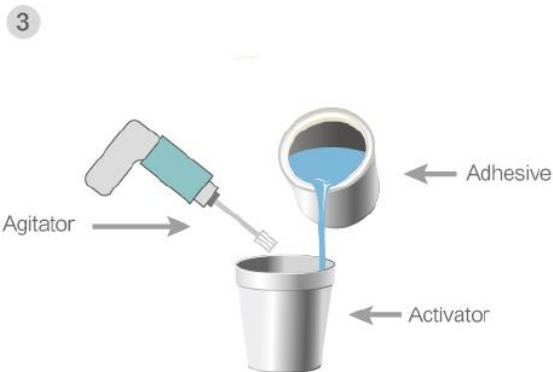
Figure 3. Take out the fully soaked fiber cloth. Mix the adhesive
